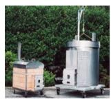
Japan, China and Australia innovated producing biochar in small pyrolysis ovens like those on the left. Great for residential use, these units dispose of waste, generate heat and power and produce biochar for the family garden. Stoves bigger than these can be converted to mobile units and taken to the biomass source saving on transportation costs when large amounts of biomass are available periodically but not regularly in a specific location.
